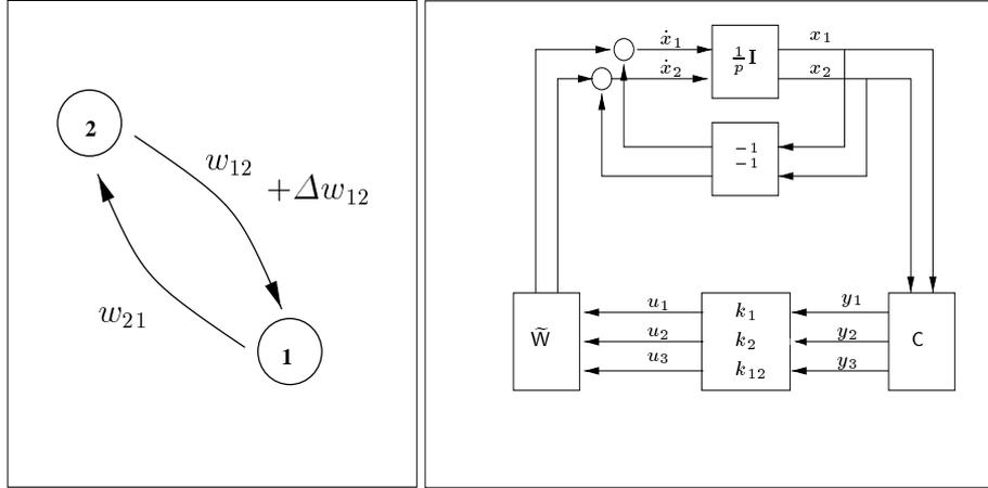
**Fig. 1.** (a) The minimal recurrent network with time-varying weight  $w_{12} + \Delta w_{12}$ . (b) The corresponding feedback circuit according to (3) with modified weight matrix  $\tilde{W}$  and additional feedback  $k_{12}$  to account for the time-varying  $\Delta w_{12}$ .
