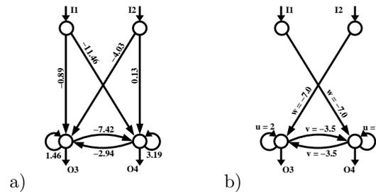
Figure 1: a) Evolved MRC with two input neurons. b) The principal structure of an MRC.
