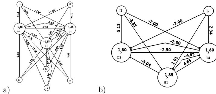
Figure 2: An evolved neural controller generating exploratory behavior with photo-tropism: a.) the full network, b) detail without light sensor inputs.
