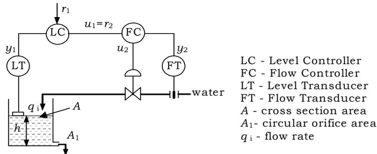
Figure 2: Schematic diagram of the level-flow pilot plant
