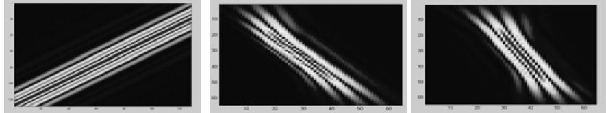
Fig. 3: From left to right: example basis function of ridgelet analysis, orthonormal ridgelet and ridgelet frame
