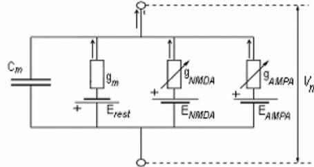
Fig. 2: the electrical circuit corresponding to synaptic conductances.
