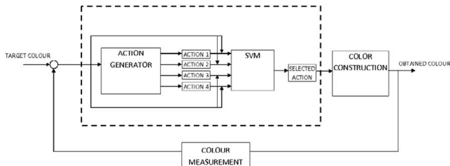
Fig. 1: Outline of the automated process: the interaction of the classifier and the actions' generator allows achieve the target colour in a loop.
