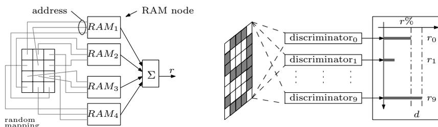
Fig. 1 – Example of a RAM-discriminator and of a WiSARD
