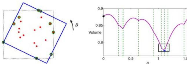
Fig. 1: 2D Oriented bounding box: the volume  $f(R)$  is not differentiable and presents multiple minima.
