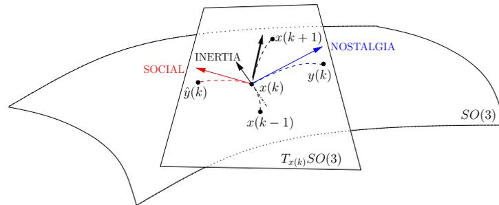
Fig. 2: Computation of the position update in the tangent space of  $SO(3)$  centered at  $x(k)$ . The new iterate  $x(k+1)$  is constructed using a combination of inertia, nostalgia and social contributions in  $T_{x(k)}SO(3)$  and is then retracted to  $SO(3)$ .
