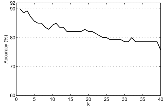
Fig. 3: Sensitivity analysis of the k value plotted against the accuracy for the supervised k -NN learning scheme.
