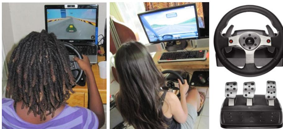
Fig. 1: The old “Tux-prototype” (based on an instrumented version of the “super-tuxkart” game) and its basic steering wheel (left), and the new “realistic-prototype” (center) and its “force feedback” steering wheel with pedals (right).
