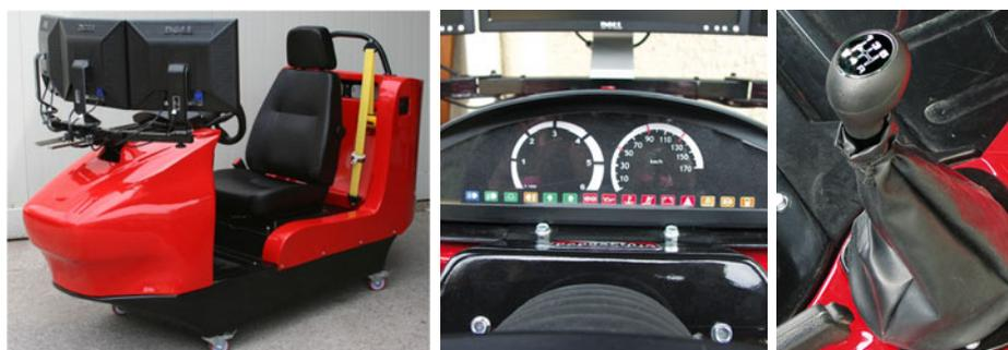
Fig. 5: The “Barracuda 2” simulator that ApportMédia should soon make available for our research, with the same software as for our realistic-prototype, but with a gear shift, handlebar controls, a parking break, and a familiar dashboard.
