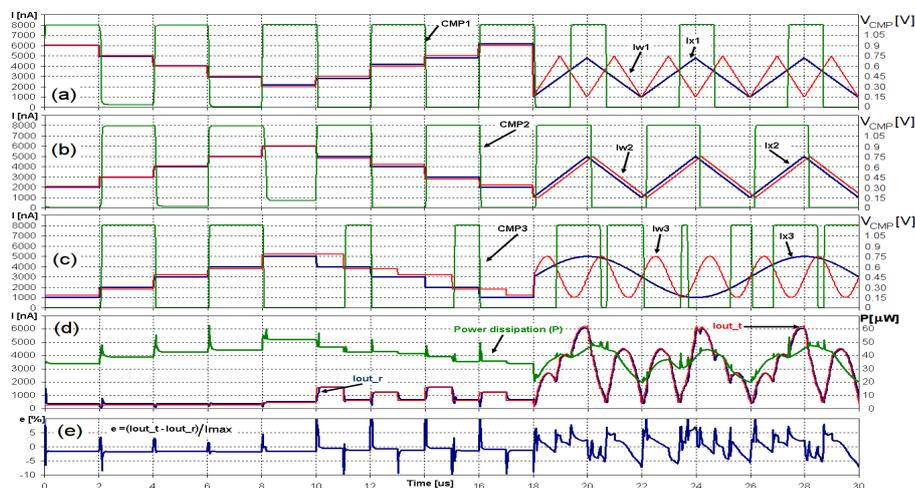
Fig. 3: Verification of the DCC at the transistor level for large currents in the range of 1–6  $\mu\text{A}$ : (a, b, c) Input ( $I_x$ ), weight ( $I_w$ ) and the comparator output signals, (d) Theoretical ( $I_{\text{out},t}$ ) and real ( $I_{\text{out},r}$ ) DCC output current and the power dissipation, (e) Error:  $I_{\text{out},t} - I_{\text{out},r}$  in reference to maximum range of  $I_{\text{out}}$ . The DCC output current is normalized – divided by the number of inputs.
