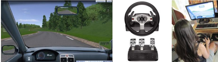
Fig. 1: The “realistic car simulator software” (left) have been used with a Logitech G27 and its “force feedback” steering wheel with pedals (centre), and was used to collect low level data related to the subjects behaviour in the simulation (right).
